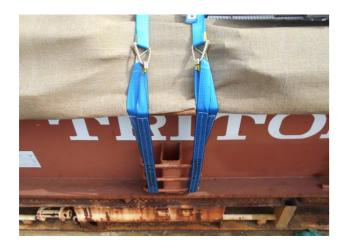
To address this costly issue one eye of the axel strap is passed through the lashing point and the two eyes connected to the hook and keeper on the ratchet which is then tensioned resulting the ratchet being in gauge.
